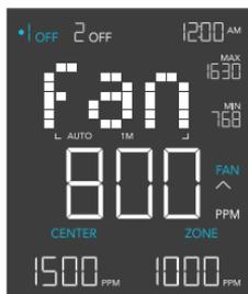
The set zone value is the buffer around your set center value that is equal to half its setting. (ex. 1000ppm. Buffer zone is 1000-2000ppm).
