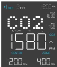
The set zone value is the buffer around your set center value that is equal to half its setting. (ex. 400ppm. Buffer zone is 1000-1400ppm).
